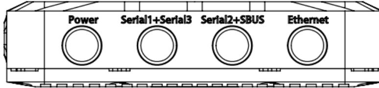
The device has four data ports, power ports from left to right, serial ports 1 and 3, serial port 2/SBUS, and one 100 Mbit/s network port. Air@link supports wi-fi connection. You can configure parameters or view parameters instead of using network ports.
